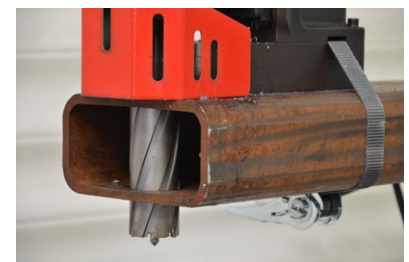
Starting point of milling up to 50 mm (2") below a level of a drill base
