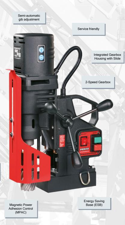
PRO 51 is equipped with the latest generation of electromagnetic energy saving base (ESB) with magnetic field shape control system (MFSC) and magnetic power adhesion control module (MPAC), which detects adhesive force of electromagnetic base and protects both the machine and the operator from work on too thin workpieces.
